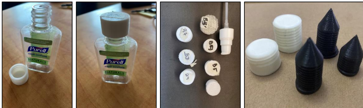
Figure 9: Threaded cap designed and manufactured for a sanitizer bottle. Right figures show test thread prints with sub-optimal thread clearance and/or pitch.
