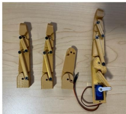
Sample 1: Prosthetic finger design using three fourbar linkages in series.
