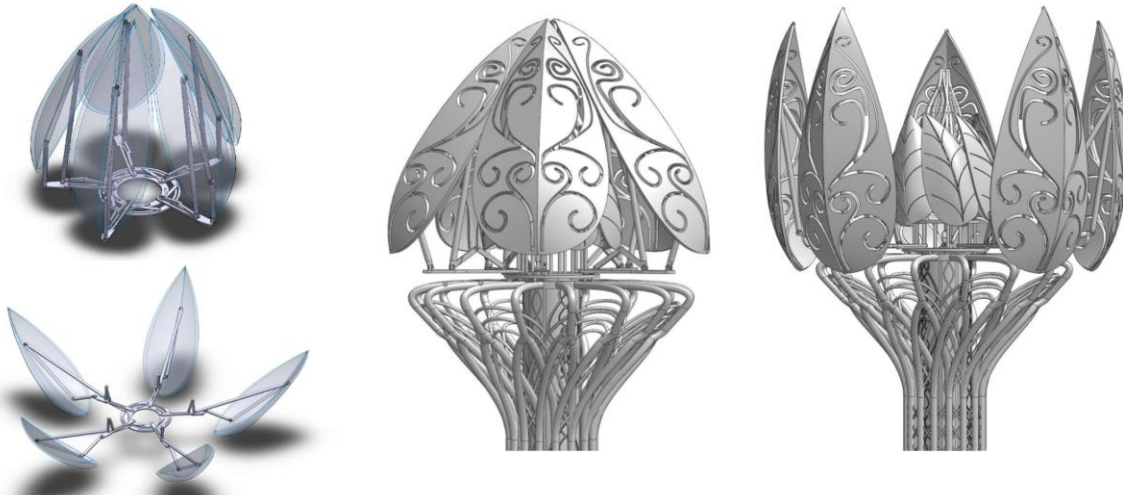
Sample 2: Sunrise alarm clock to gradually light up the room, operating with fourbar linkages combined with slider joints. Inspired by the unsuspecting time scale of plant movements.
