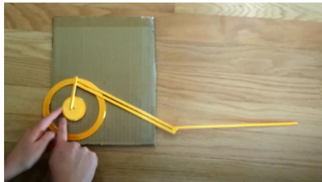
Sample 3: Ornithopter kite design, inspired by flapping motion of wings to generate lift.
