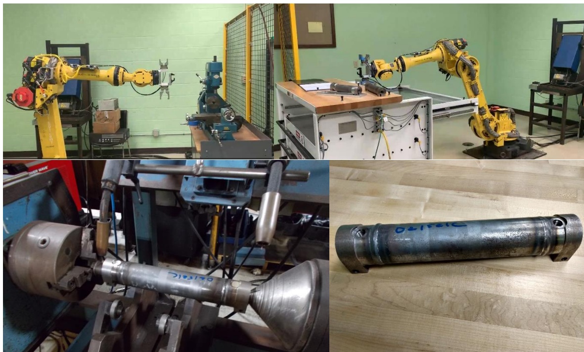
Figure 1: Equipment used in Project 1, including a drawer, lathe machine, Fanuc robot, stamper, and other accessories.
