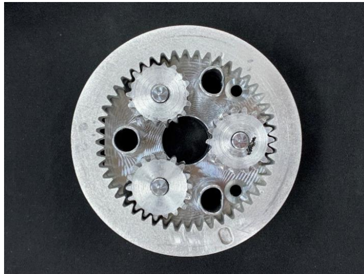
Fig. 14 Cast gears used in a planetary gear set for the capstone project.
