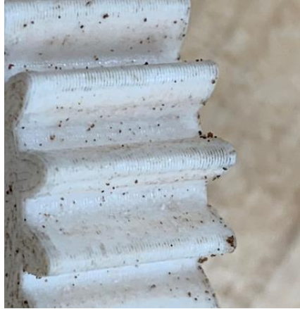
Fig. 3 Sample part filament printing layer lines.
