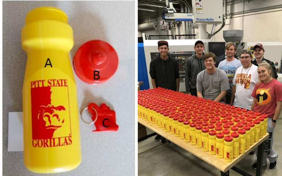
Figure 3: Left: A) Blow-molded bottle with screen printed decoration, B) Injection molded bottle lid, and C) Gorilla keychain made from discarded cup holders. Right: Students at a PET Production Party.
