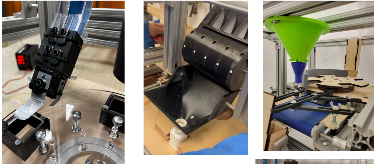
Figure 4. Examples of student team proof-of-concept prototypes built from 80/20 stock parts, laser- and hand-cut wood, 3D printed parts, and fiberglass forms. Clockwise from top-left: substation for dispensing and placing the cap, funnel and indexed cylinder for pill filling, transition from rotary index table to conveyor belt, complete bottle filling monoblock.
