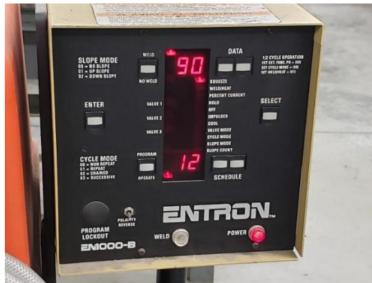
Figure 3: The welder controller set to program 12.
