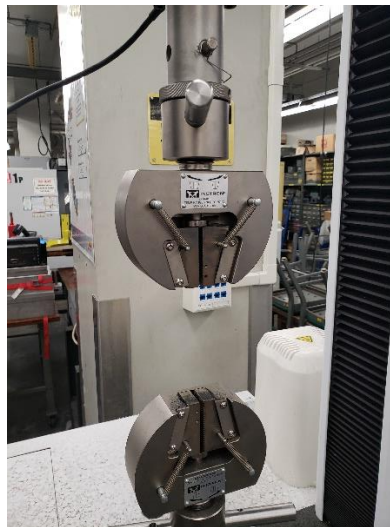
Figure 6: Clamps used to hold the pieces and pull them apart.
