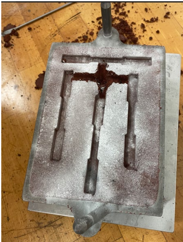
Figure 2 (L): Match plate for sand casting; figure 3(R) Sand Mold
