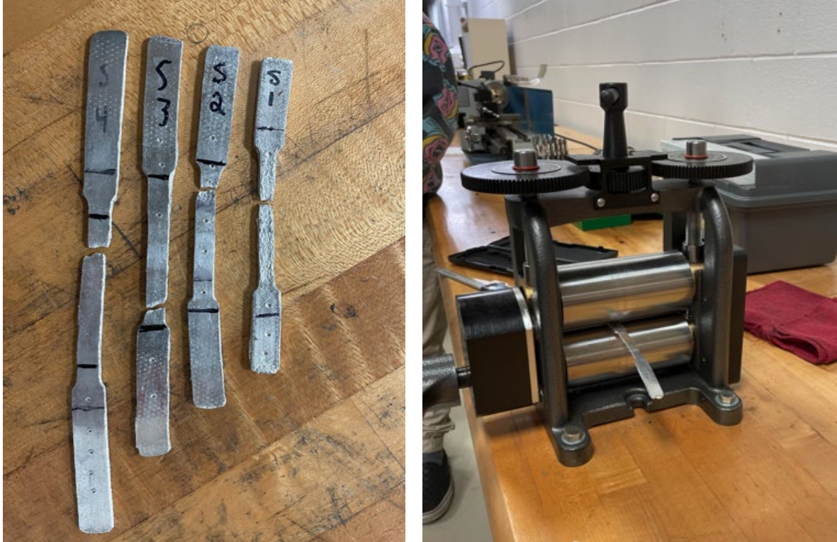
Figure 6 (L): cold-rolled specimens after tensile tests; Figure 7 (R): Specimen in cold rolling
