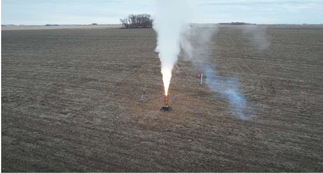
Figure 3. The largest motor ever designed and built at Iowa State was developed by the Cyclone Rocketry propulsion team and produced over 800 pounds of thrust.
