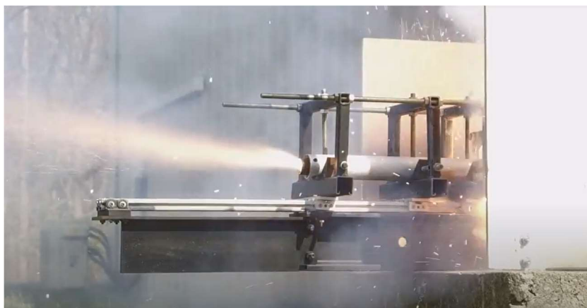
Figure 6. One of the propulsion team's early failures on a subscale motor.
