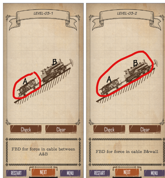
Figure 3: Level 03-1 shows car A isolated to find the force between the two bodies (left), and Level 03-2 shows both cars, A and B, included in the system (right).
