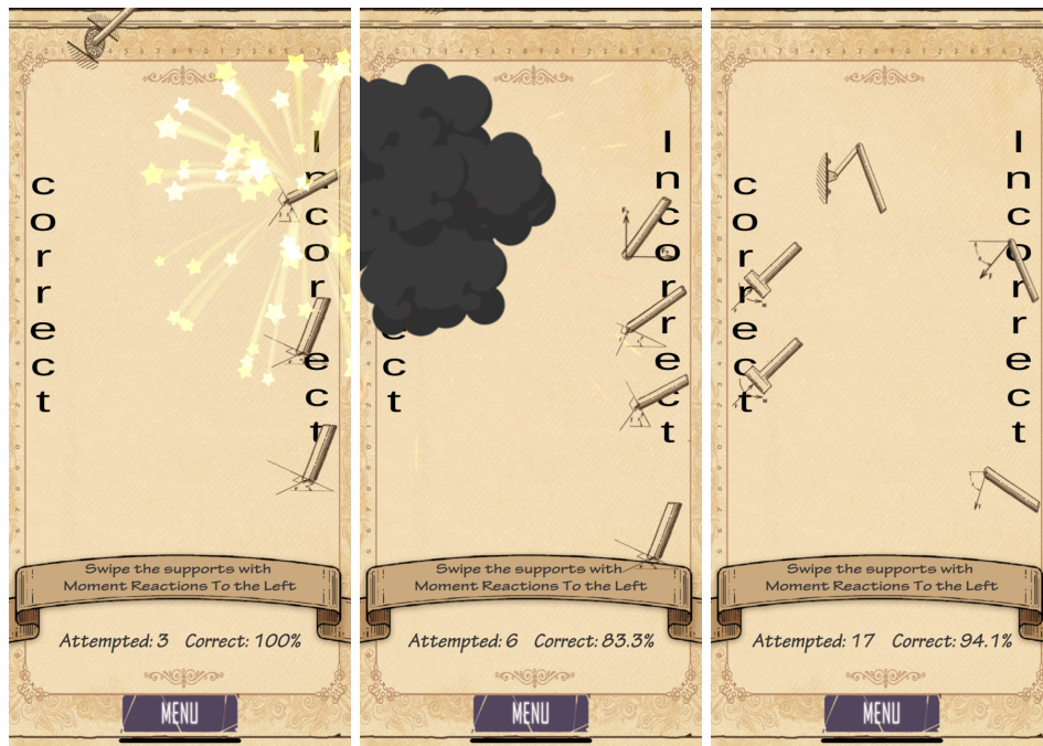
Figure 4: A roller correctly identified as having no moment reaction (left), a pin misidentified as having a moment reaction (center), and connections before and after swiping (right).
