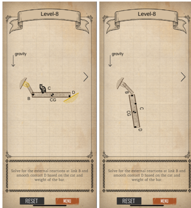
Figure 5: A weightless link and smooth contact support beam BD (left). Upon clicking the link, the system simulates the swinging of beam BD when supported by only the selected link (right).
