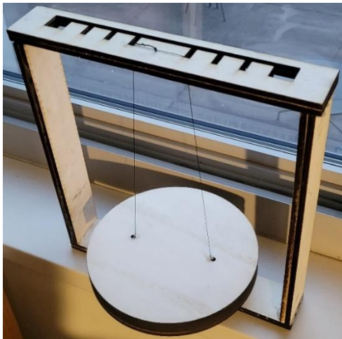
a. Student A’s set-up achieving 0.4 % error when a = b .
