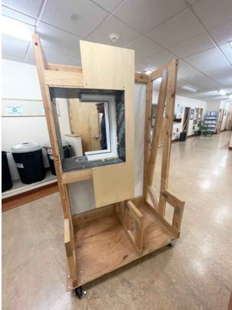
Figure 2. Images of integrated truss system framework demo. Photo by Todd Nicewonger, 2022.
