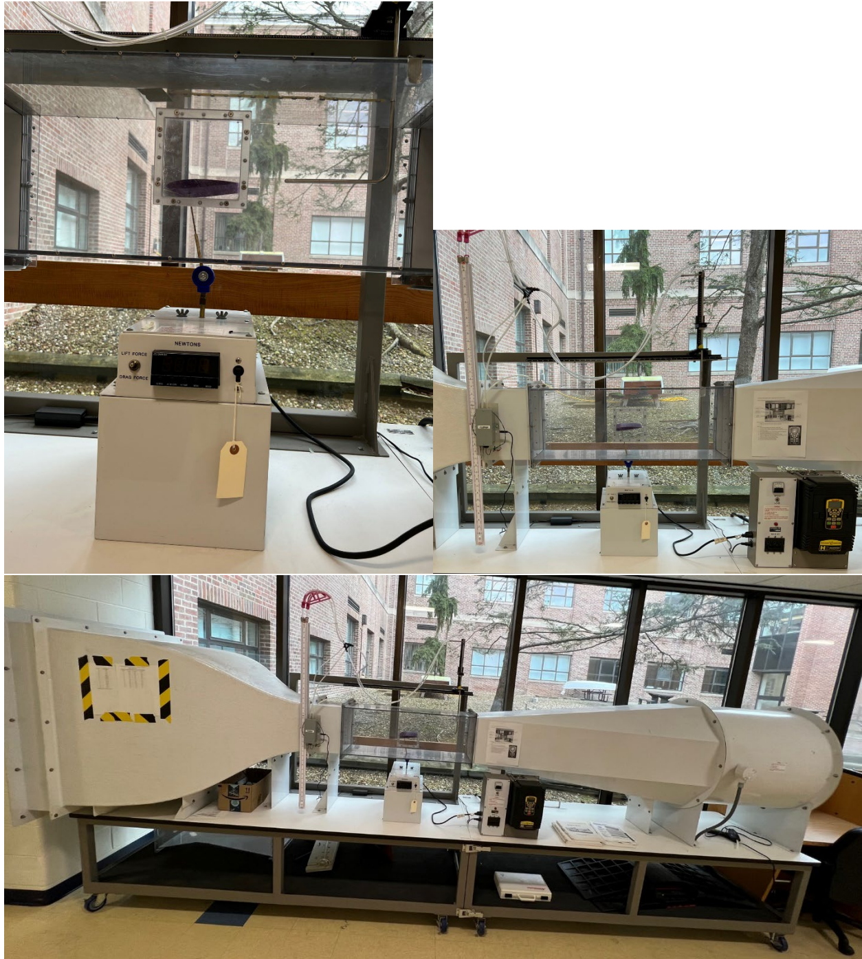
Figure 2: Hampden H-6910-12-CDL Wind Tunnel with 5-inch chord-length airfoil loaded at -15^\circ angle of attack. The Wind Tunnel has a pitot-static tube, manometer, and lift/drag load cell. Clockwise from top left: airfoil loaded on the load cell that reads both drag and lift data; the full test section with manometer and pitot-static tube behind the airfoil; full wind tunnel. Flow is left to right.
