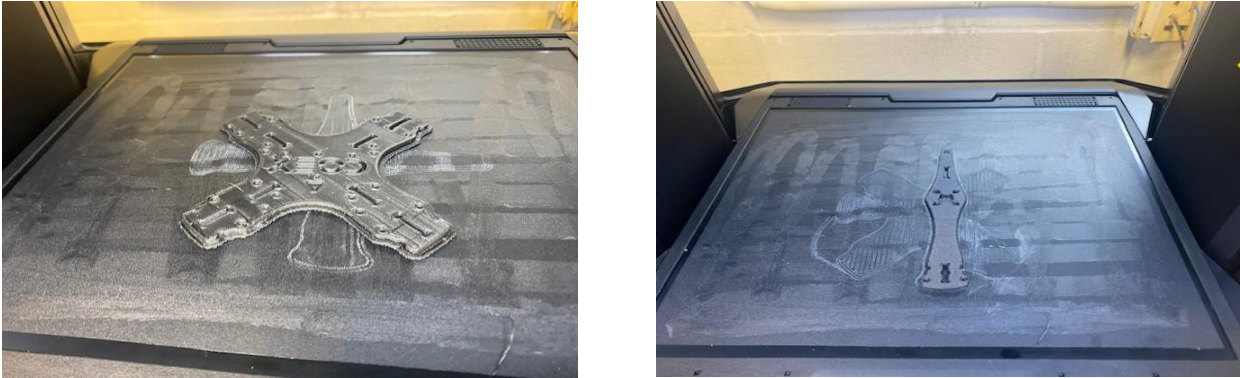
Fig.6: Prototyping the parts of the COEX Clover drone by 3D printer
