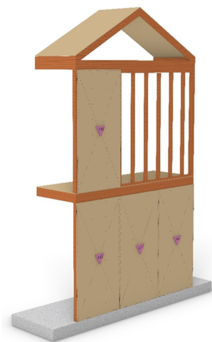
a) Partially Assembled Shear Wall
