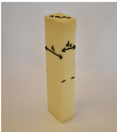
Figure 2. Column Buckling Model
