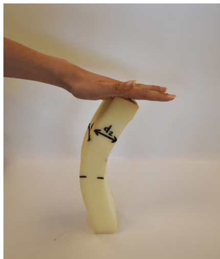
a) Weak-axis Buckling
