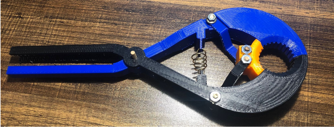
Figure 8. 3D printed product to test the functionality of the final design before sending for final production [4]
