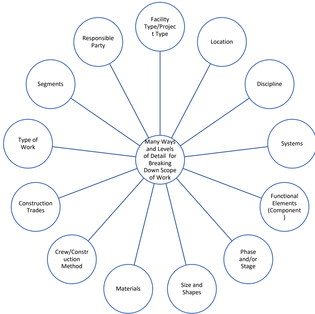
Figure 3. Options for grouping, detailing, aggregating, and breaking down the project scope of work.
