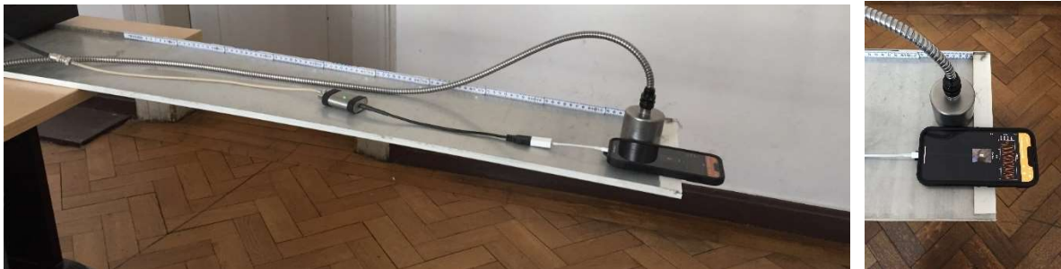
Figure 1. Experimental setup #1 with iPhone 13 Pro and PCB accelerometer at the tip of a flexible cantilever.
