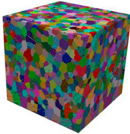
Figure 2. Simulated grain morphologies of Ti-6Al-4V alloy
